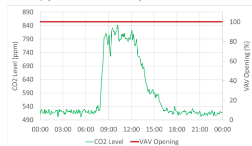
Figure 13: CO 2 level and VAV opening in room U181 on 29 November
